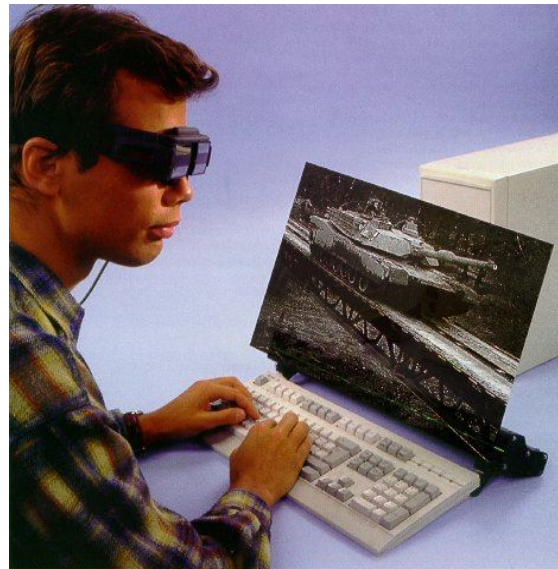
Figure 10: Active Stereo Display Example Using Shutter Glasses Source: Authors' Archives
