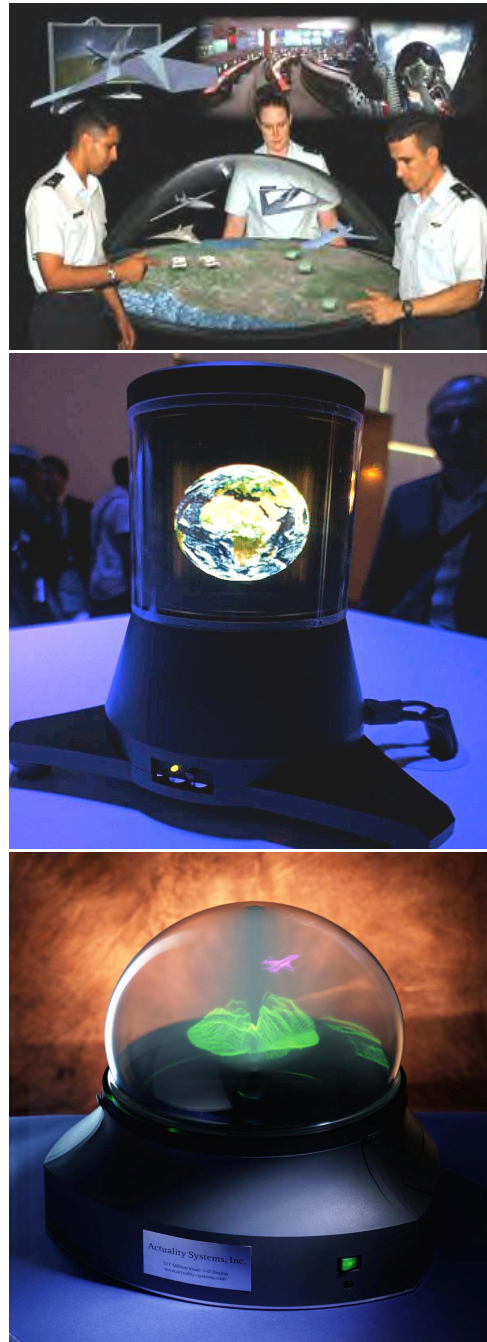
Figure 12: A concept C 2 Volumetric Display (Upper), Sony Ray Modeler (Middle) and Actuality Perspecta Volumetric Display (Lower) Sources: Authors’ Archives and www.gizmodo.com
