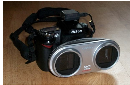
Figure 5: Loreo 3D Lens for Digital Cameras. Source: www.denverslair.co.uk
