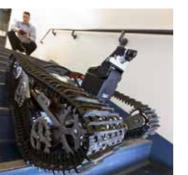
The mobile manipulator will also be used to deploy a pipe-climbing robot (developed by KAERI), which can scale the complex pipework that fills many nuclear installations. Such robots could be used to enter Fukushima or parts of old nuclear plants in order to locate, model, monitor, cut and remove contaminated legacy plant parts.
