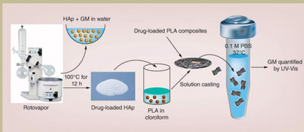
Figure 2: Schematic representation of the drug loading and release method used in the work.
