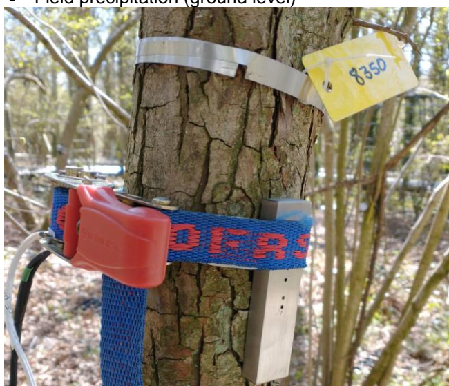
Sue Quick fits small Tranzflo compensated heat pulse probes to Hawthorn trees measuring xylem sap flows for her BIFoR FACE tree-soil-water relations research.
