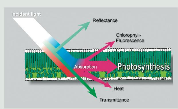
How light energy falling on a leaf is partitioned. About 78% of the incident radiation is absorbed, while the rest is either transmitted or reflected at the leaf's surface. About 20% is dissipated through heat and only 2% emitted as fluorescence, as a by-product of photosynthetic reactions occurring within the leaf itself. Mapping Photosynthesis from Space - a new vegetation-fluorescence technique. ESA Bulletin 11/2003 116:34-37.
