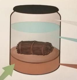
Mesocosms simulate real-life scenarios under controlled conditions. Here they are used to investigate the impact of wood in river sediments on biogeochemistry.
