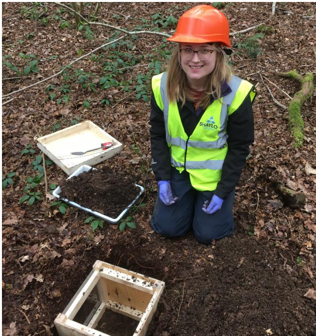
Dr Michaela Reay installing root box for accessing roots for exudate collection under FACE Underground project
