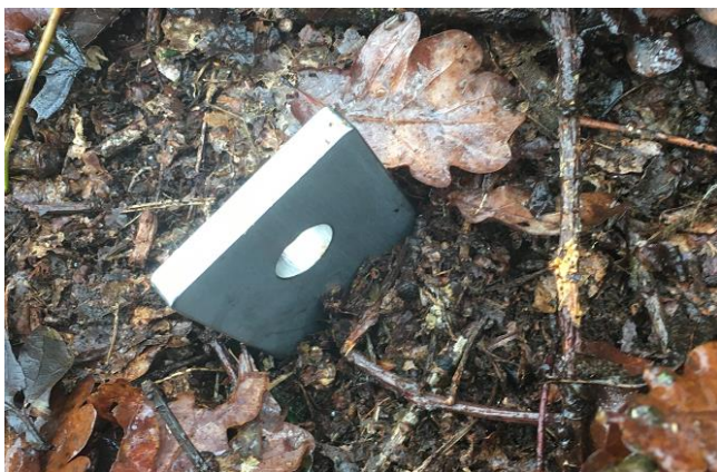
Manon Rumeau a new PhD student has joined the QUINTUS team for research on biological N fixation and mineralization under elevated CO 2 fumigation. This is one of many ion exchange resin probes she has helped to install.
