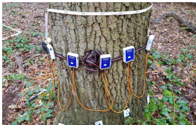
Tomography of an oak stem to search for cavities; work carried out in support of Sue Quick's PhD studies on plant-water relations under elevated CO 2 .
