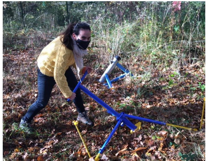
Dr Marie Arnaud demonstrates the slanted coring device that is used to insert minirhizotrons into the soil. Minirhizotrons allow images of fine roots to be captured over a season so that root productivity can be measured.
