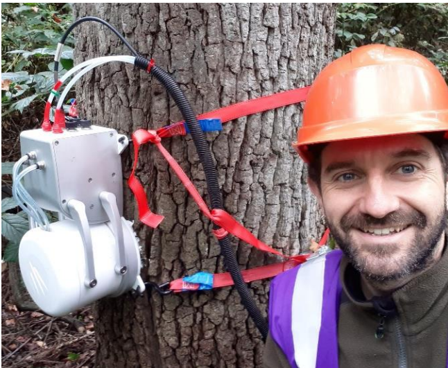
Dr Joseph Barba Ferrer demonstrates kit to measure the diffusion of CO 2 and methane into/out of an oak stem.
