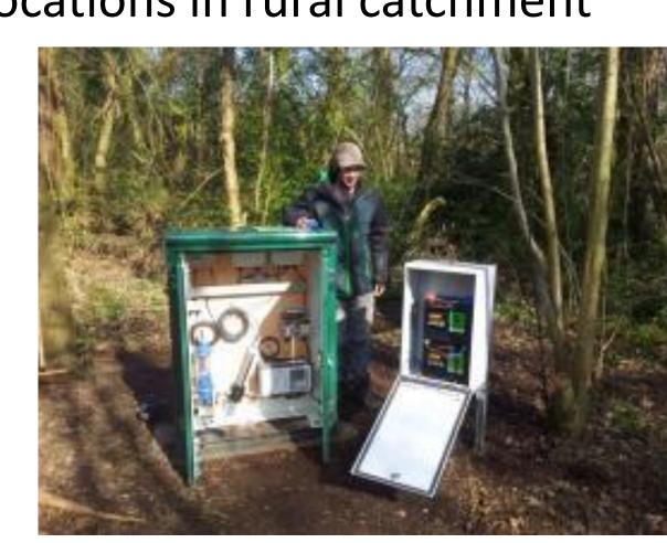
In-situ water quality monitoring station (optical, fluorescence, absorbance) (top) Mill Haft catchment with mixed landuse, currently undergoing shift to sustainable agriculture (left)
