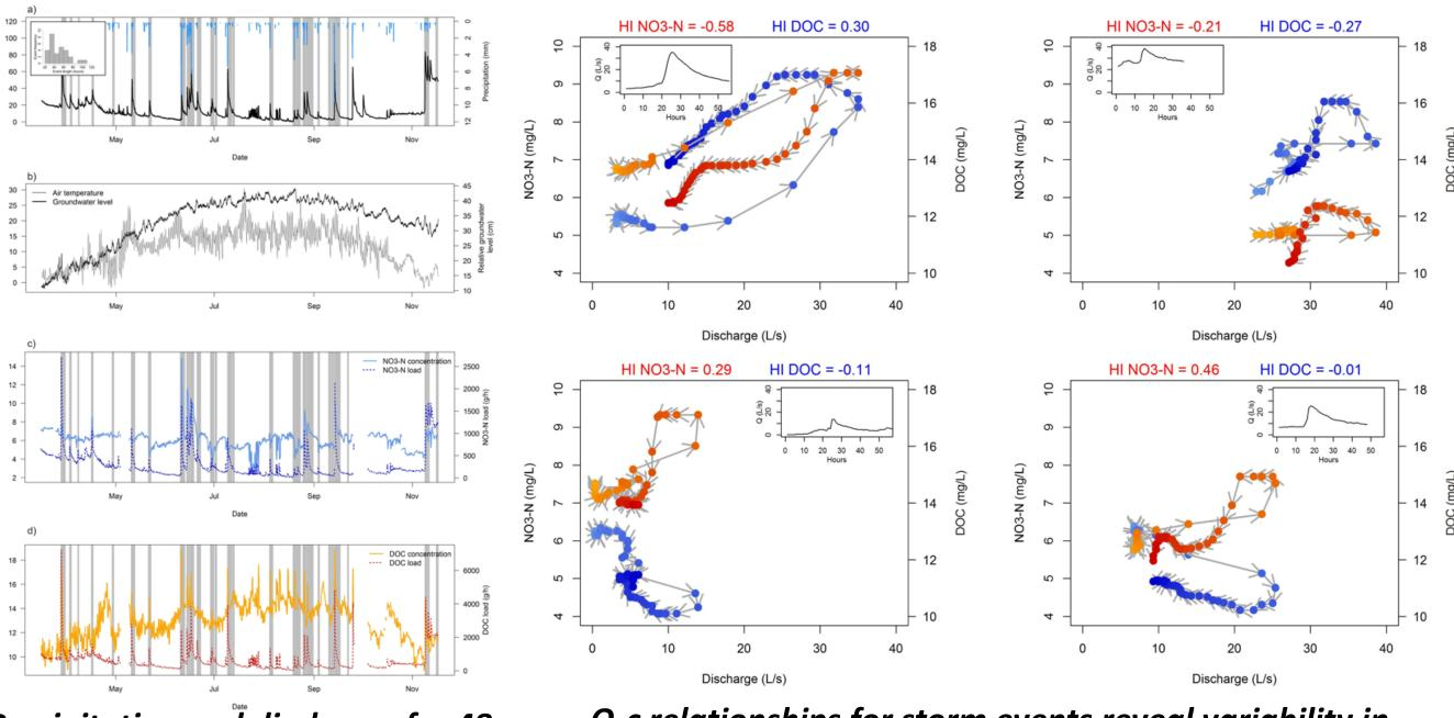
Precipitation and discharge for 48 selected storm events with corresponding NO<sub>3</sub> and DOC concentrations
