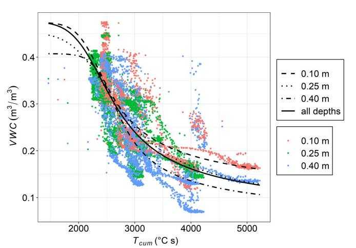
Soil depths and transect specific A-DTS soil moisture calibration - comparison to TDR/FDR point observations along both slopes
