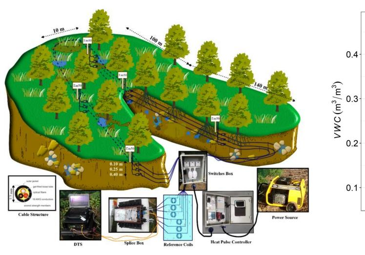
Experimental setup of A-DTS soil moisture monitoring, comprising three soil depths along two 250m hillslopes, 25 cm sampling resolution
