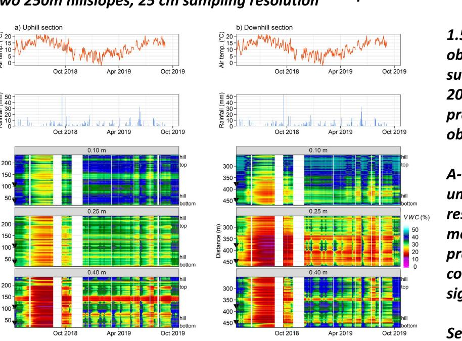
1.5 years of A-DTS soil moisture observations, including substantial summer drought in 2018 as indicated by precipitation and temperature observations (top)
