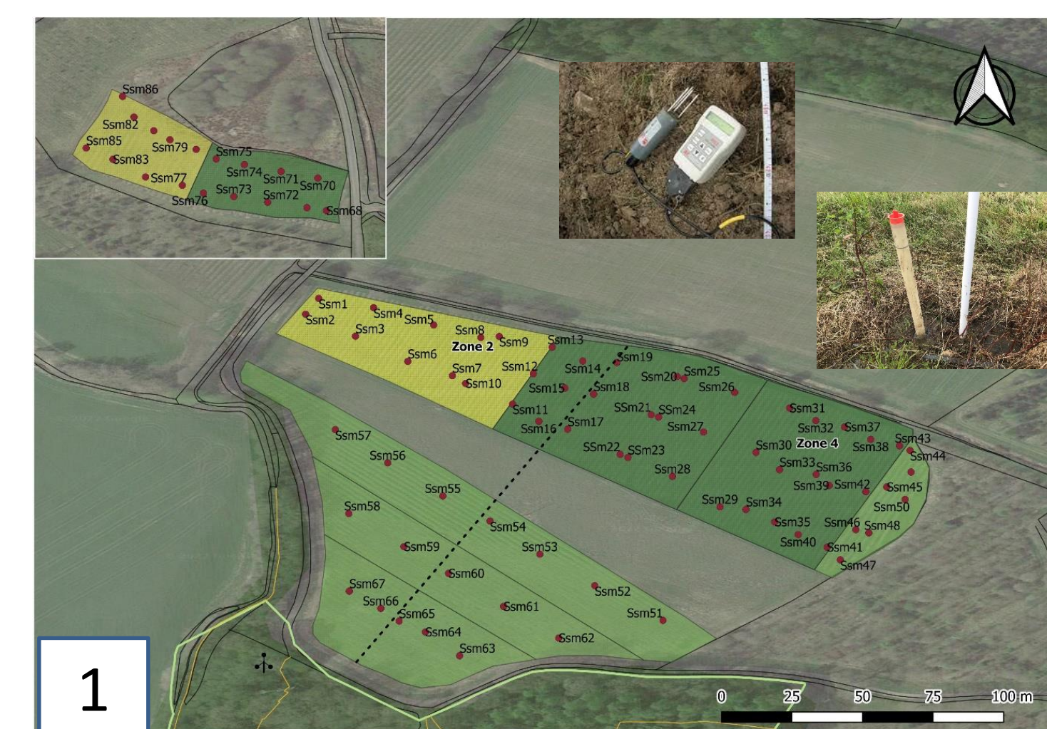
1 Experimental setup to acquire data on superficial (5 cm) and deep soil moisture (10,20,30,40 cm) on weekly time resolution.
