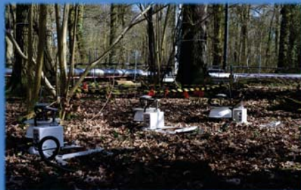
Figure 1: Long-term chambers deployed on top of collars installed in the soil measuring soil respiration. Each array has three plots and each plot has a surface collar, a collar with 41µm window and with 1 µm window
