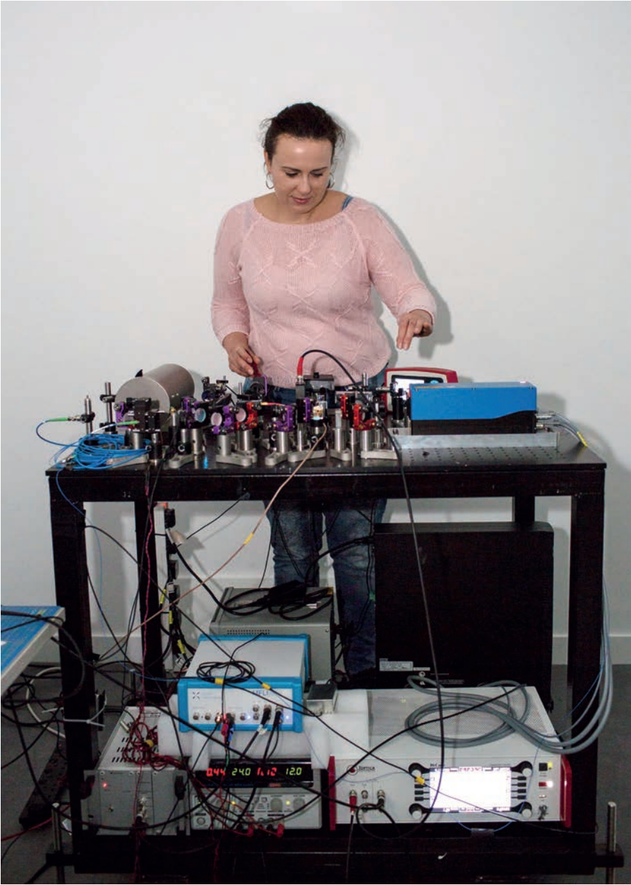
Anna Kowalczyk testing the prototype for the first in-house OPM sensor developed at the CHBH
