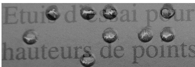
Figure 11 Examples of cracking on Braille dots in height condition 6
