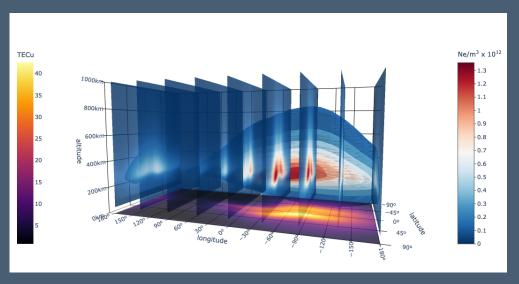
3D surface plot of the ionosphere electon density (red/blue colormap) with a 2D contour plot of the vertically integrated electron density (purple/yellow colormap)
